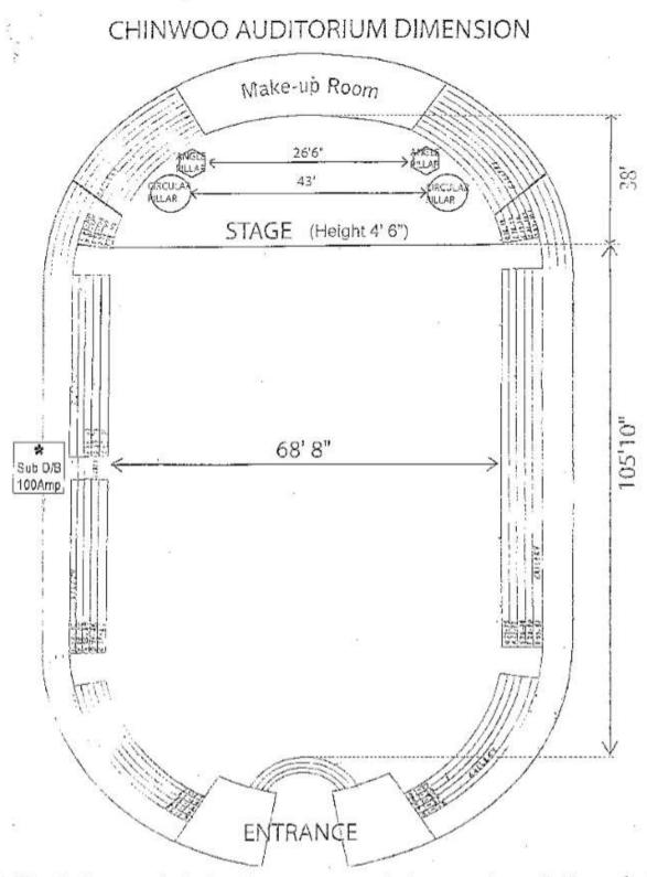
\* The 3-phase and single-phase power sockets are only available and located at the Sub D/B (max. 100A), for indoor use only.
